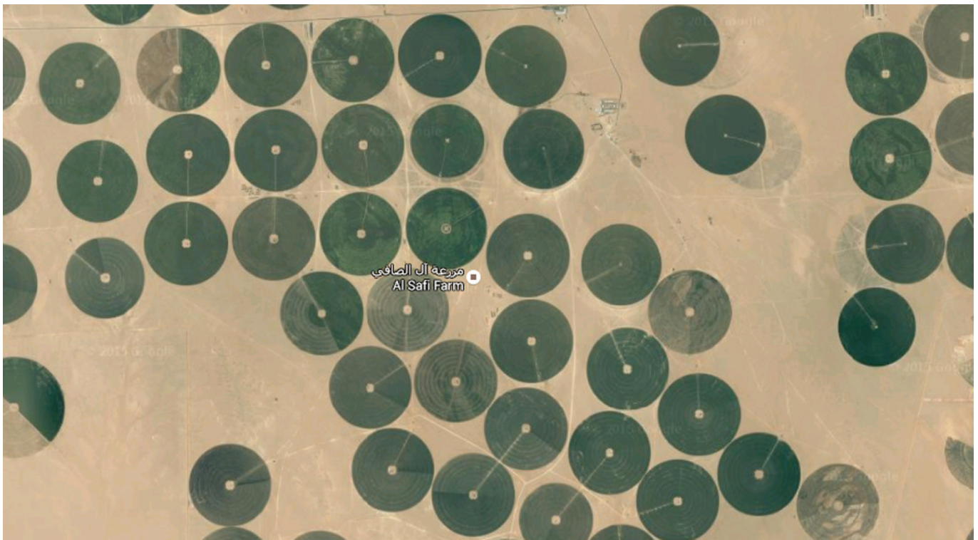
Fig. 14 - Fields irrigated with the center-pivot system at the Al Safi Farm (Saudi Arabia) (source: maps.google.com).
